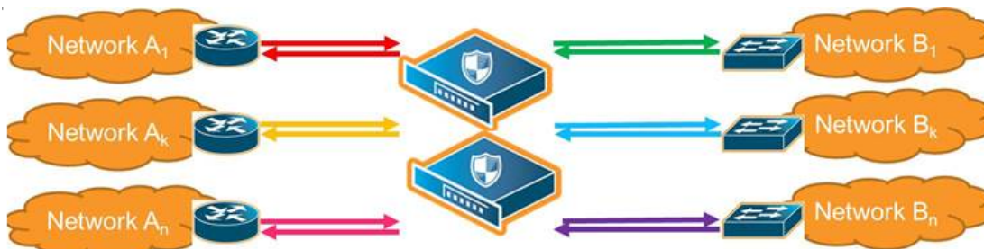
Figure 70 Inline Tool Inserted in Multiple NetA-NetB Links
